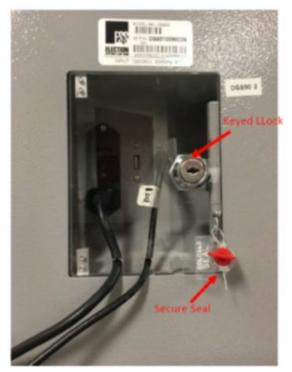
(d) On the right side of the DS850, three clear access doors protect the USB ports. The access doors must be secured using the integrated key locks and wire or padlock seals.
