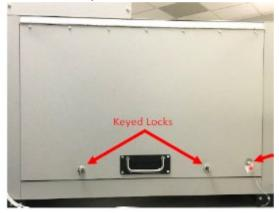
(c) On the left side of the DS850, a clear access door protects the power switch, power cord, network port, and USB port. The access door must be secured using the integrated key lock and a wire or padlock seal; and
