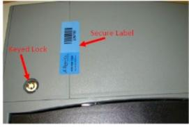
(e) Close the touch screen display and secure the lock with a medium barrel key. Affix a label seal vertically over the place where the main section of the unit meets the touch screen display; and
