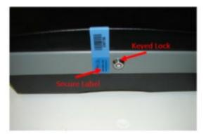
(f) Affix a second label seal over the seam where the top of the unit joins to the base;
