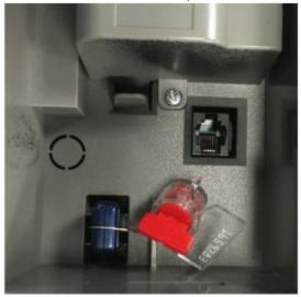
(d) Ensure that the rear access door is locked with a medium barrel key and affix a label seal over the place where the rear access door meets the body of the machine. The rear access door covers the backup USB flash drive;
